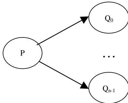
Module P produces a stream of elements with interdeparture time  $T_p$ . For  $i = 0 \dots n-1$ , let  $T_i$  be the ideal service time of  $Q_i$ , and  $p_i$  the probability that an element is sent from P to  $Q_i$ , with  $\sum_{i=0}^{n-1} p_i = 1$ .
